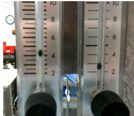
Some generators systems separate the Hydrogen from the Oxygen. Picture shows ratio of 2 to 1
